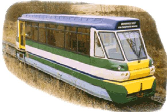
Now, frankly, it was a bumpy ride in parts because of the freight-only track and because the four wheels, close together are not on a sprung bogie, but the next development, specially planned to be trialled on the Wensleydale line will be a bit like a 'bendy-bus' with sprung bogies.
